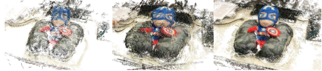
Figure 10. SLAM based dense reconstructions. Left: reconstruction from direct SLAM cameras; Middle: reconstruction with only camera refinement. Right: the proposed method with both camera refinement and dense alignment.
